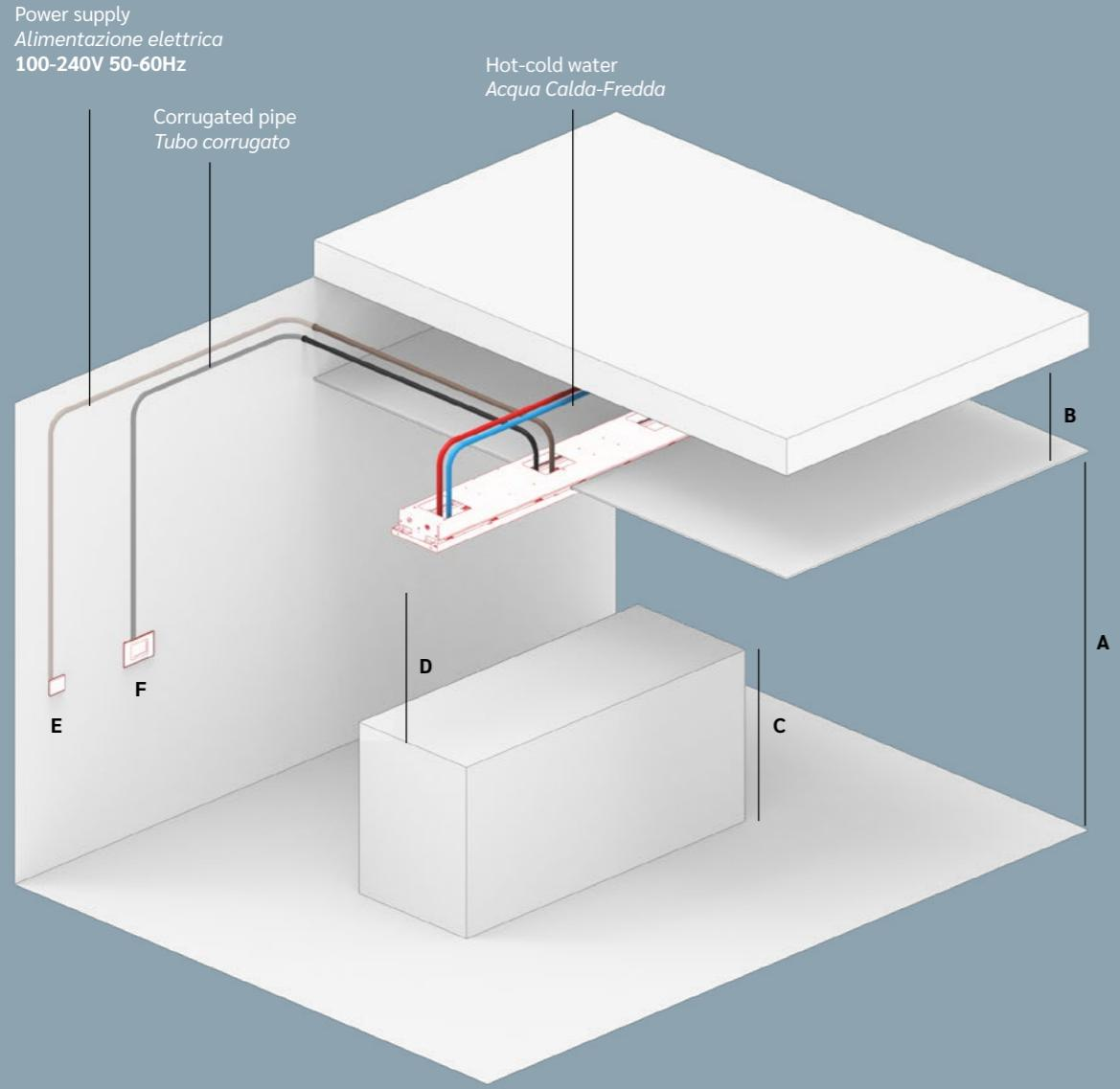
**A:** Floor / false ceiling distance: Variable according to the type of fixing
